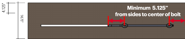
UNDERSIDE TOPPER VIEW
